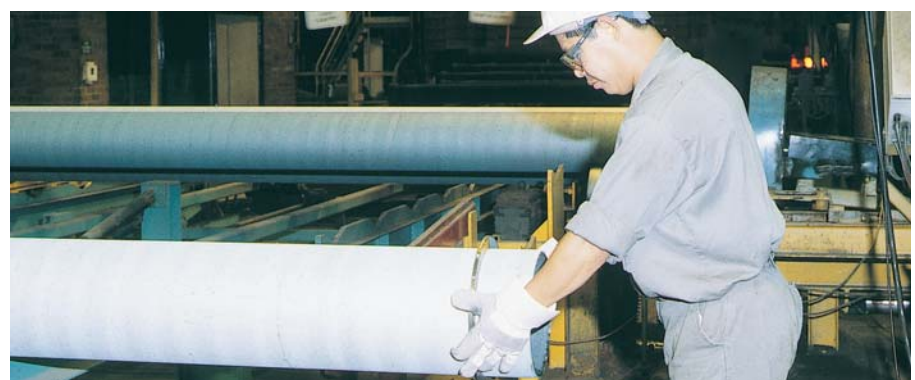
In-line dimensional checking
